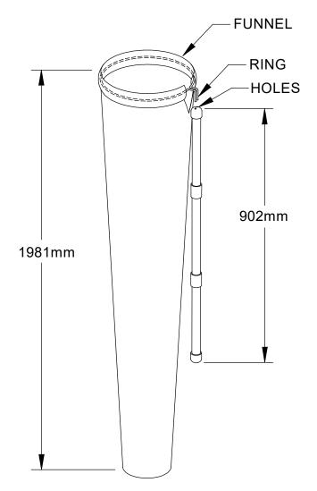
THE MODEL 190.95.90.90 SHOWER TEST KITS GUIDE THE WATER TO A FLOOR DRAIN OR CONTAINMENT BUCKET.
